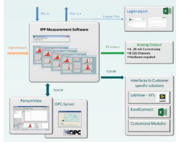
IPP – This is the core measurement interface, designed to control the Parsum probe measurement process and provide a clear presentation of the results.
