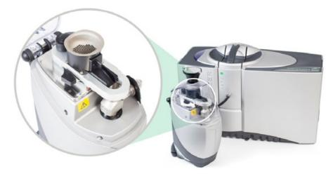
When measuring the particle size and size distribution of bulk materials, dry powder dispersion is advantageous as it enables the analysis of a large mass of powder. This helps when sampling materials which are polydisperse, improving result reproducibility and assisting detection of out-of-specification materials. In addition, dry powder dispersion eliminates the need for liquid dispersants, reducing the cost of measurement compared to wet dispersion analysis.
