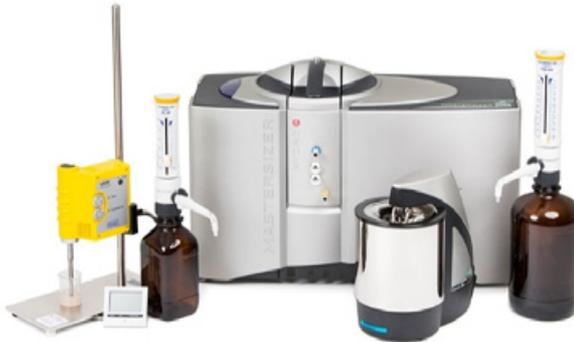
The Mastersizer 3000 Chocosizer kit provides for fast, reliable chocolate particle size analysis as part of routine process and quality control. It includes all the components required for chocolate sample preparation and measurement using the Mastersizer's Hydro MV or Hydro SM dispersion units, including:
