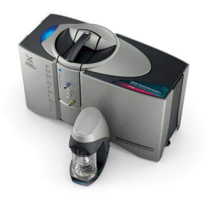
The Hydro EV has a unique dip-in centrifugal pump and stirrer design that achieves full and rapid dispersion in standard laboratory beakers, allowing close matching of the dispersant volume to the application requirements. Following measurement, the dispersion head can be raised out of the beaker, enabling quick cleaning and sample recovery.
