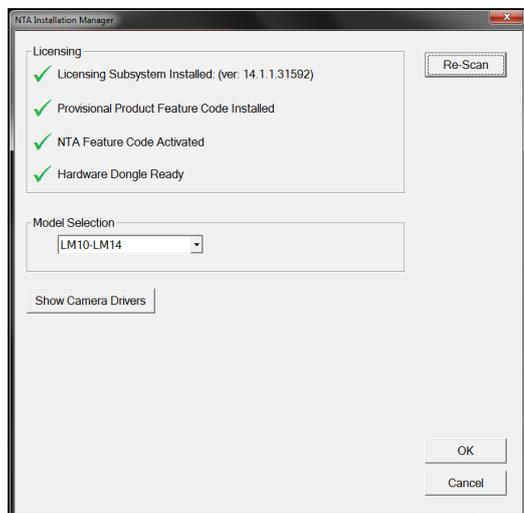
The NTA Installation Manager controls security, model selection and camera drivers. When upgrading NTA 2.3 to NTA 3.0 all license features should show a green tick with the correct instrument model selected.
