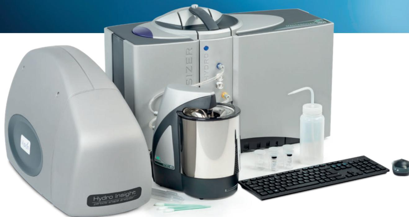
The Hydro Insight accessory provides this – combining Vision Analytical's dynamic imaging expertise with Malvern Panalytical's flow cell technology. Sitting alongside our Mastersizer 3000 laser diffraction system, the Hydro Insight provides real-time images of your liquid particle dispersions
