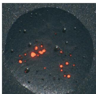
Uncoated Be exposed to a 1 M HCl solution shows many corrosion holes (orange dots) within 30 minutes.
