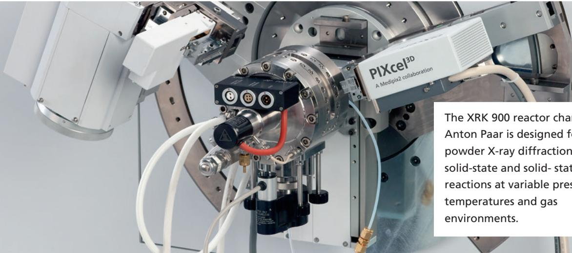
The XRK 900 reactor chamber from Anton Paar is designed for *in situ* powder X-ray diffraction studies of solid-state and solid-state gas reactions at variable pressures, temperatures and gas environments.
