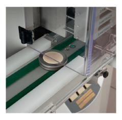
The press unit is fitted with a 30-position sample carrousel in order to be able to announce a whole batch of samples. The complete automation is controlled by PANalytical's SamTracs control system.
