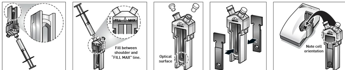
Figure 1: Wetting, filling and insertion of the folded capillary cell
