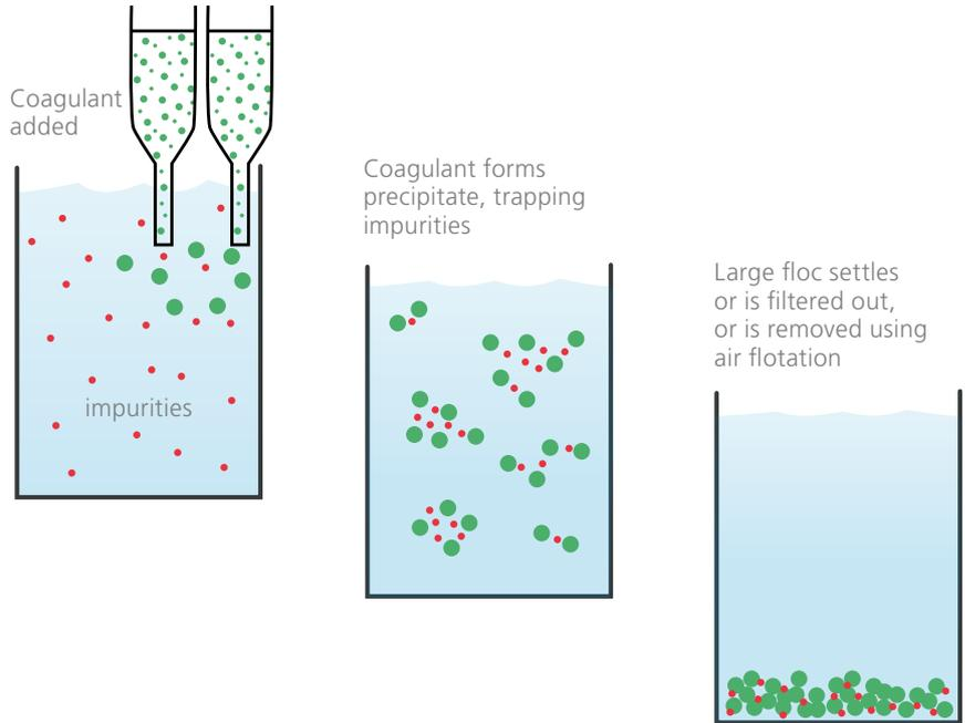
Continuously measuring the zeta potential of water following coagulant dosing:
