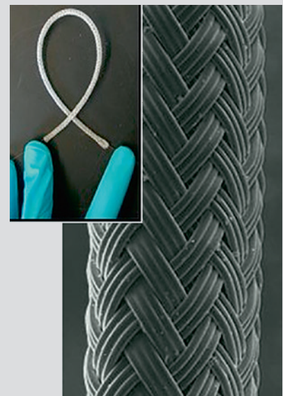
Fibers braided into guidance conduits for nerve regeneration
