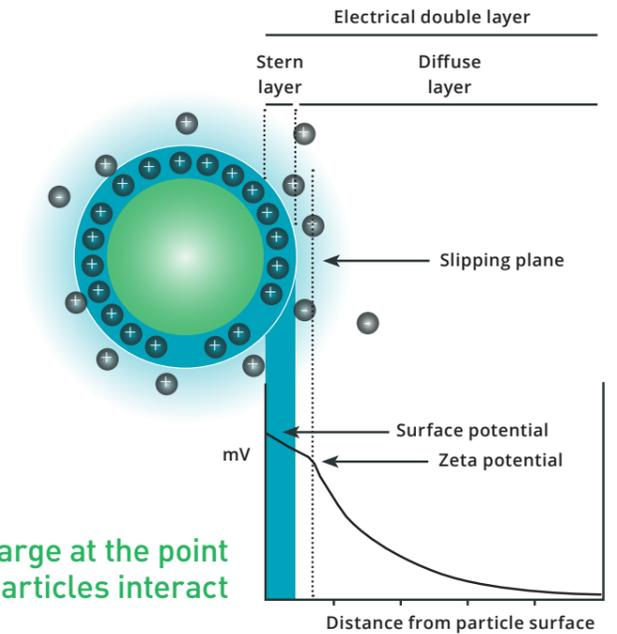
Zeta potential is the charge at the point where suspended particles interact
