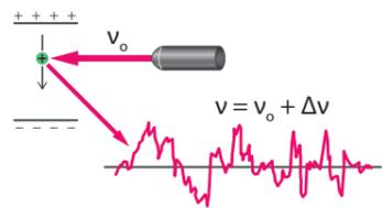
Zeta potential measurement using a laser
