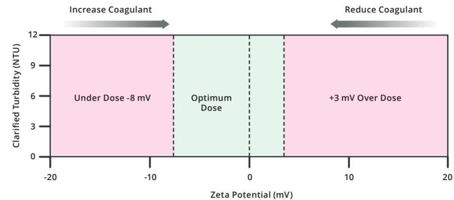
Continuously measuring the zeta potential of water following coagulant dosing:
