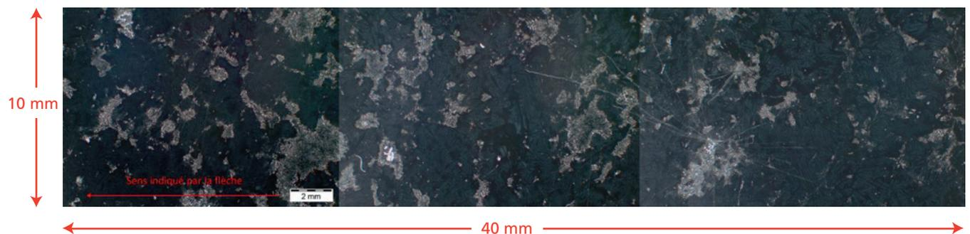
Figure 2. Scanning electron microscopy (SEM) micrograph, highlighting the surface of a slab sample after etching. White regions indicate segregation of Cr, Ni and Mo from the bulk.
