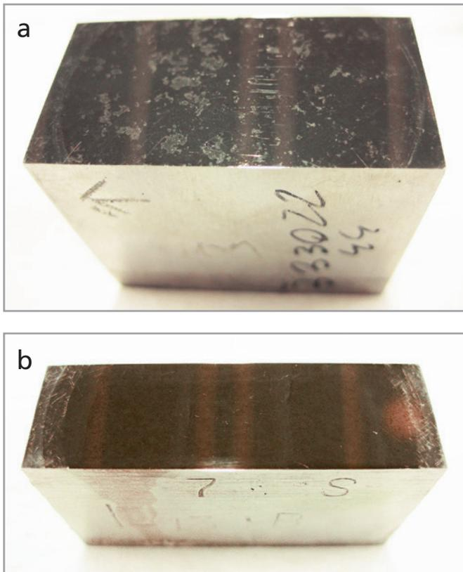
Figure 3. a) Sample Brame 1 analyzed for a 6.5 mm x 11.5 mm mapped area; b) sample Brame 2 analyzed for 10 mm x 11 mm mapped area
