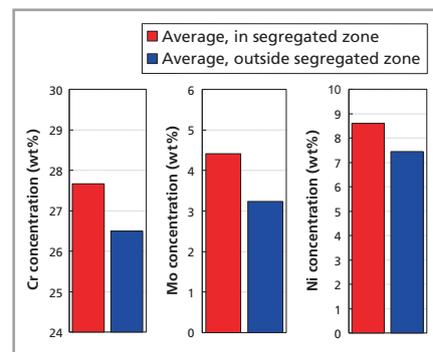
Figure 1. Variations in Cr, Mo and Ni concentrations between bulk slab and segregated zones occurred at casting
