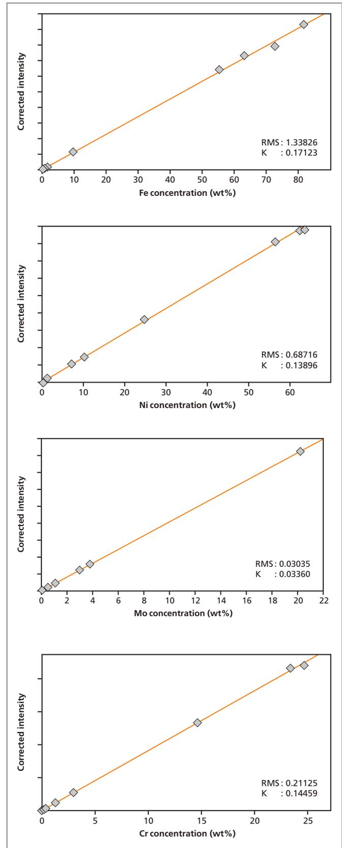
Figure 4. Calibration lines on 0.5 mm spot size for Fe, Ni, Mo and Cr
