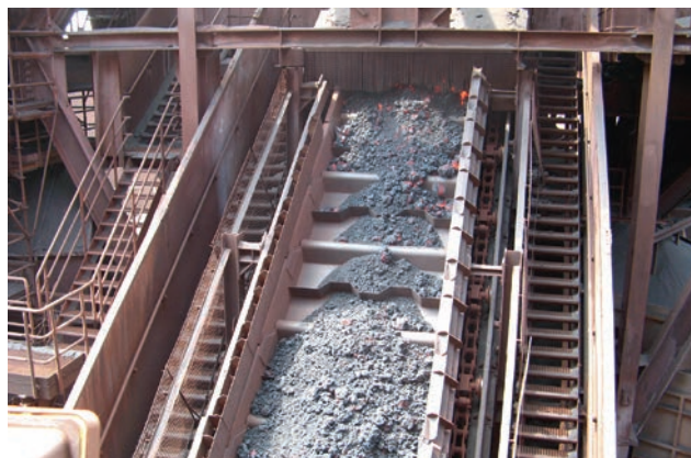
Figure 2. Hot sinter is transported into the sinter coolers.
