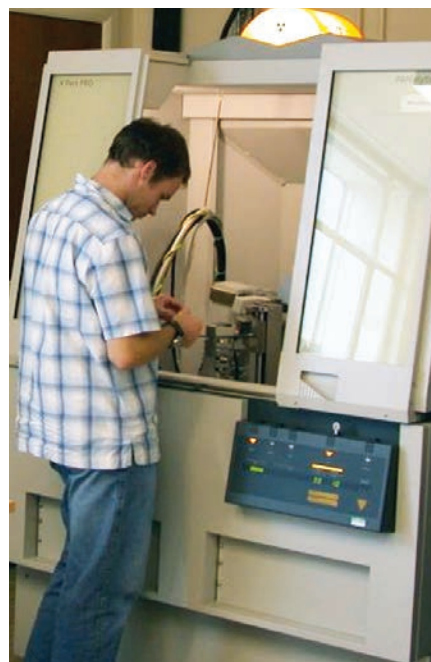
X-ray diffraction equipment at Amgueddfa Cymru - National Museum Wales. This enables rapid, and non-destructive analysis of a wide variety of specimens.
