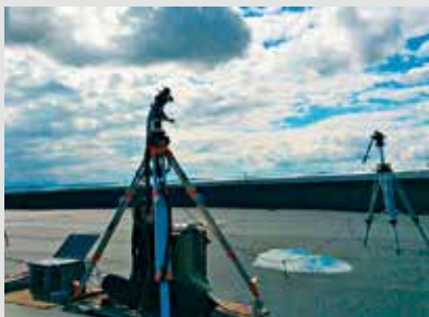
Figure 2. An example creating more accurate simulated skies using a custom sky scanner, paired with an ASD FieldSpec instrument
