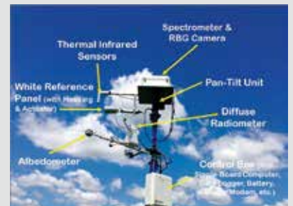
Figure 4. Components of the EcoSpec system (collecting white reference data before every data collection from the land surface, at each position around the tower, so that hyperspectral data is accurately converted to reflectance values). The spectrometer in this setup is an ASD FieldSpec 4. 3
