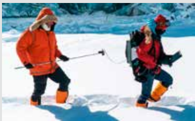
Figure 1. Innovative use of an ASD pistol grip to measure light being reflected off snow (left, with fiber optic cable accessory) and sand (right, with fore optic accessory) 1
