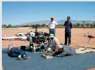
Figure 3. An ASD instrument on a UAS / mini-helicopter for the purpose of collecting airborne remote sensing measurements 2
