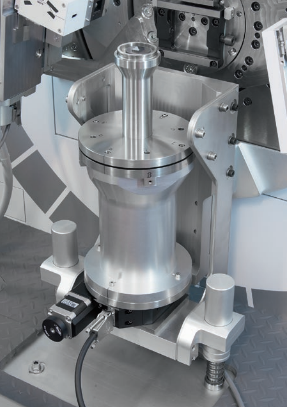
Jig for orienting large single crystals prior to cutting and polishing
