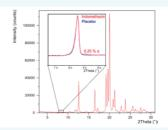
0.25 w% of alpha-Indomethacin in a formulation of 5% gamma-Indomethacin in a lactose based formulation.
