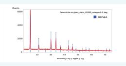
A 36 min GIXRD measurement of a MAPbBr3 Perovskite layer deposited on a glass substrate.
