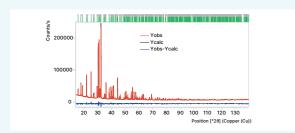
Rietveld refinement of synthesized and heat-treated AgCaVO4, Ref: G. Nénert, Z. Kristallogr. 2017; 232(10).
