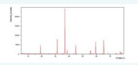
Co3O4 measured with Copper radiation on an Aeris with 1Der detector.
