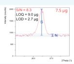
7.5 µg of Quartz on a silver mesh. Measured in 6 minutes. A signal to noise ratio of 8.3 is achieved. With this measurement speed 9 micrograms quartz are above the limit of quantification (NIOSH 7500).
