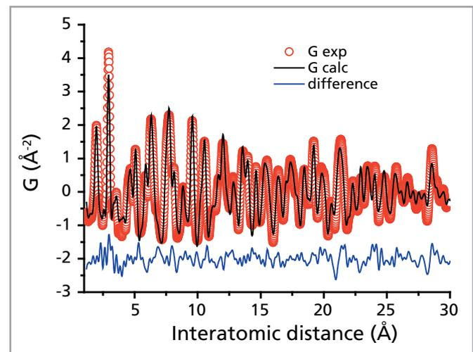
Pair distribution function measurement of material electrode using Ag radiation (data taken from E. Talaie et al., *Energy Environ. Sci.*, 2015, 8, 2512-2523)
