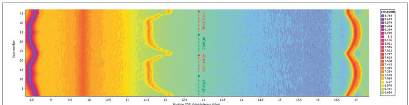
Variation in the XRPD data during two full charge and discharge cycles. The peaks at about 8.5° and 17° 2theta belong to the LiNMC phase, (003) and (101) reflections respectively. The peak at about 12° 2theta is the (002) reflection of graphite.
