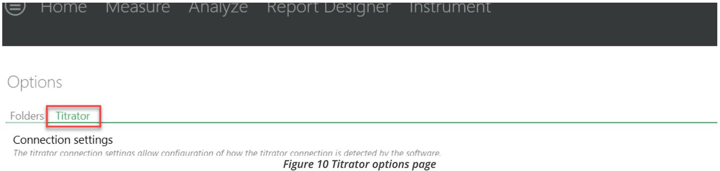
On the COM Port drop down menu, select USB Serial Port (COMXX) as shown in figure 11. (Note that the COM port number and description may vary). If the titrator has been detected on this port, then a green tick will be visible See *Figure 11*.
