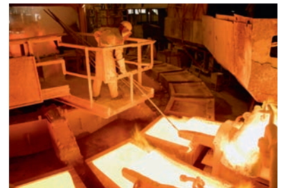
Casting of copper anodes in the casting carousel
