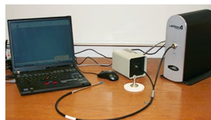
Setup for data collection using the ASD LabSpec® 4 benchtop analyzer with a bifurcated fiber optic reflectance probe
