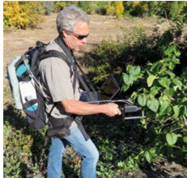
The ASD FieldSpec® 4 spectroradiometer used in situ to measure soil and crop constituents
