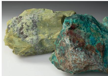
The photograph shows two different copper ores from one deposit in Peru: a light green primary sulfidic ore and a blue green secondary oxidic ore. Because of the different mineralogy and distinct processing (flotation or leaching) it is of utmost importance to separate the ore types and waste rock as early as possible in the process. In order to achieve this separation in the most cost-effective way, various technologies and their combinations are available.
