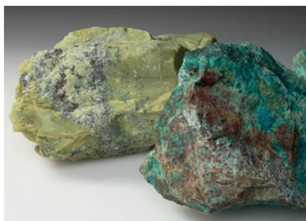
The photograph shows two different copper ores from one deposit in Peru: a light green primary sulfidic ore and a blue green secondary oxidic ore. Because of the different mineralogy and distinct processing (flotation or leaching) it is of utmost importance to separate the ore types and waste rock as early as possible in the process. In order to achieve this separation in the most cost-effective way, various technologies and their combinations are available.
