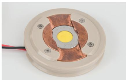
undergo a phase transition during charging and discharging cycles, XRD can provide a wealth of information on the condition of the battery in operando. PANalytical has developed a number of different sample holders for batteries to support this type of analysis.
