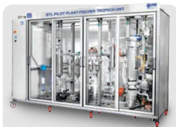
Biomass reactor then FT to synthetic fuels
