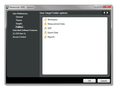
Again, hover over the shortcut and click on the pencil icon in order to change the target directory. Note that this is the only place in the software where the target directories can be configured when using the Basic software for the Mastersizer 3000E.
