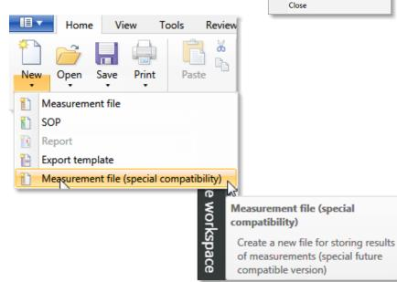
a file in the same format used by v3.20 and v3.30, select the **Measurement file (special compatibility)** option when creating a new measurement file:
