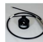
**Rapid Analysis Probe** – The Rapid Analysis Probe is useful when fast and convenient measurement is necessary or a 'lower temperature illumination' is needed.
