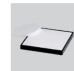
**Reference Panels** – Available in NIST traceable calibrated and non-calibrated diffuse white and gray, in varying sizes and reflectance levels and wavelength calibration panels.
