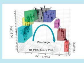
Pattern correlation cluster analysis in HighScore Plus showing various microstates the NMC cell passes through as it is cycled.
