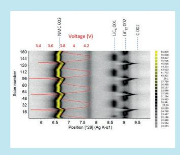
In-operando charge-discharge experiment on an NCM333 pouch cell performed on Empyrean XRD at Ambient temperature.
