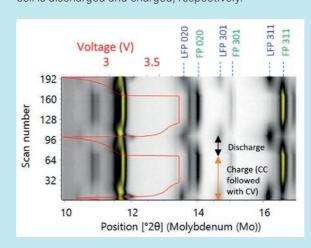
Relative concentration of triphylite (LFP) and iron phosphate (FP) phases as the cell is charged and discharged. This plot was generated in HighScore Plus software after phase quantification via automatic Rietveld refinement on the entire dataset.
