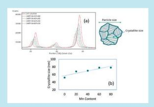
(a) XRD pattern shift with increasing Mn content in LMFP samples due to lattice expansion, and (b) crystallite size estimated in HighScore shows size increase with increasing Mn concentration.
