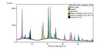
An example of Rietveld refinement on the datasets of in-operando XRD on an NMC pouch cell.
