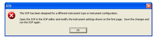
The fix for this problem is to restart the application with the instrument connected.
