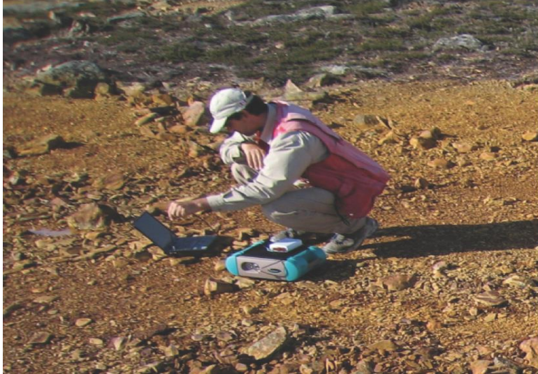
Measuring outcrop using FieldSpec Pro contact probe (calibrated halogen light source), Izok Lake area, Nunavut
