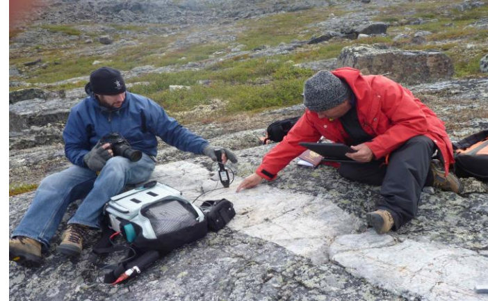
Collecting VNIR-SWIR spectra from power-washed rhyolite outcrop using FieldSpec Pro contact probe, Izok Lake area, Nunavut.
