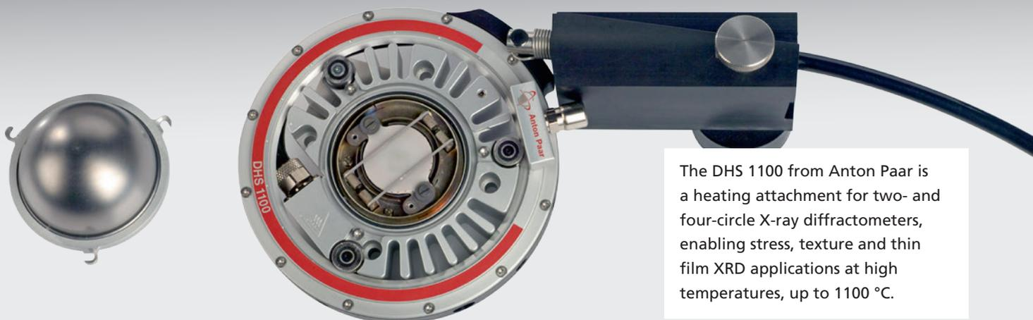
The DHS 1100 from Anton Paar is a heating attachment for two- and four-circle X-ray diffractometers, enabling stress, texture and thin film XRD applications at high temperatures, up to 1100 °C.
