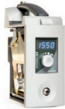
**Hydro SV** - A small volume dispersion unit designed to enable particle size analysis when dispersant use needs to be minimised or the amount of sample available for analysis is limited.
