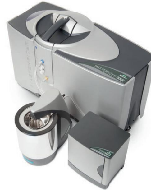
The Hydro SIGHT is a revolutionary lens-less imaging accessory for the Mastersizer range of instruments, providing rapid visualization and assessment of your liquid particle dispersions.
