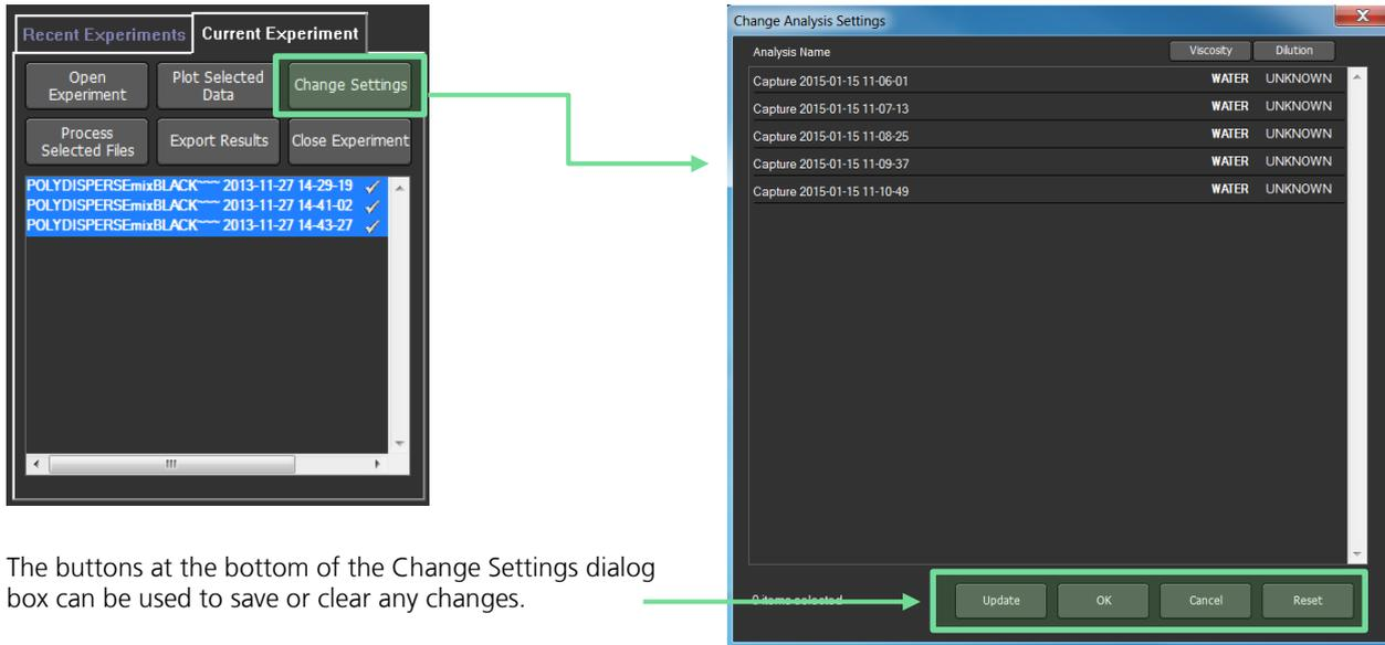
The buttons at the bottom of the Change Settings dialog box can be used to save or clear any changes.
