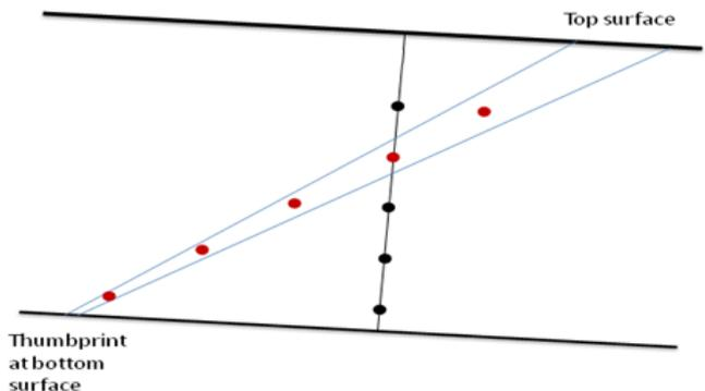
The illustration above shows the pre-set tilt to the stage and how the measurement positions correspond to different sample depths.
