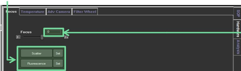
The current focus position can be changed manually by typing into the box or by adjusting the slider.
