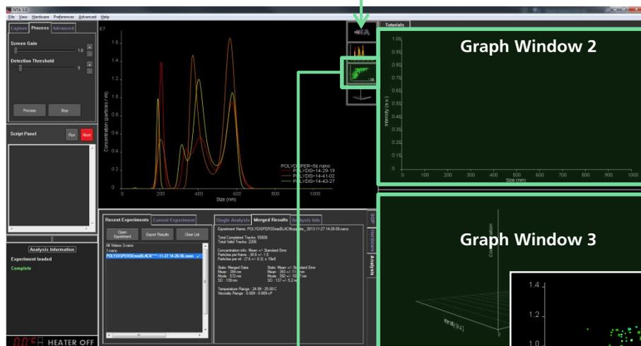
When an experiment is loaded, graph windows 2 and 3 are left empty and so can be used for any overlay plots to compare graphs between different experiments/datasets (described later in this guide)
