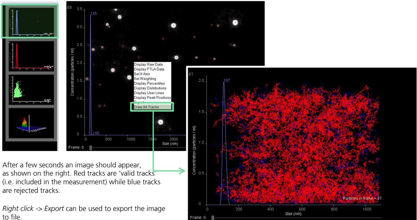
After a few seconds an image should appear, as shown on the right. Red tracks are 'valid tracks' (i.e. included in the measurement) while blue tracks are rejected tracks.
