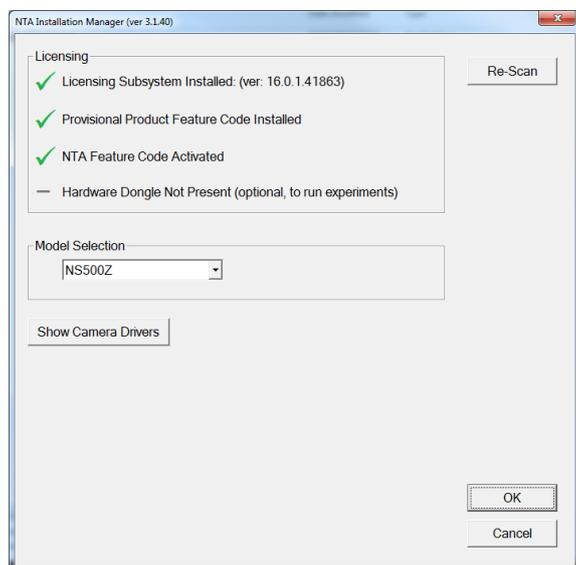
The NTA Installation Manager controls security, model selection and camera drivers. When upgrading from NTA 2.3, NTA 3.0 or another version of NTA 3.1 all license features should show a green tick with the correct instrument model selected.
