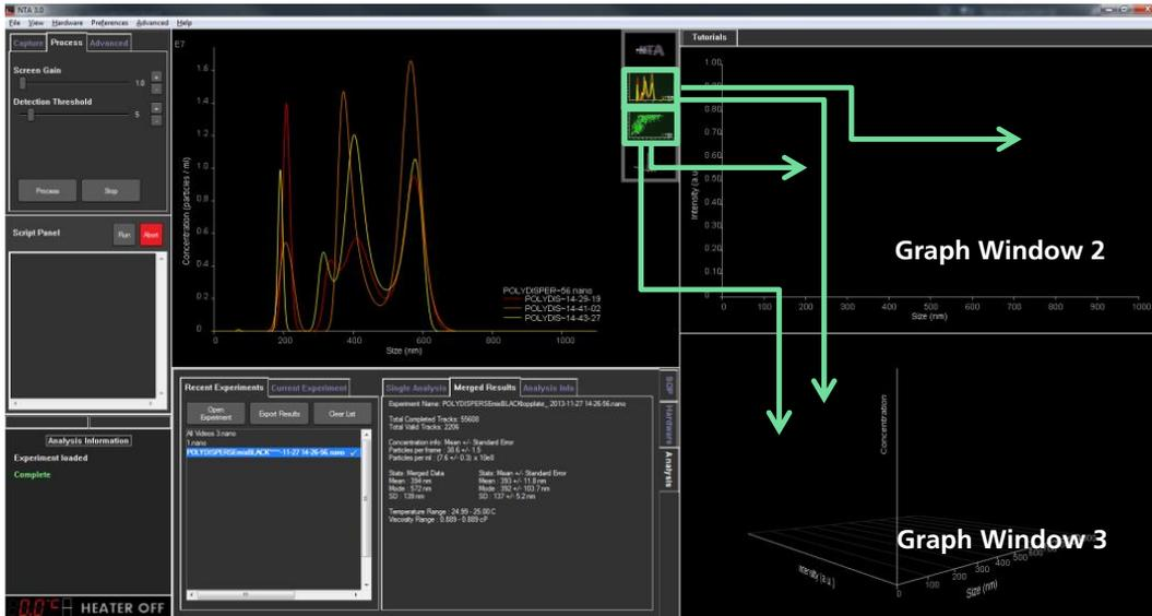
If the window that the plot is being dragged to is currently blank (i.e. on loading a new experiment), or displaying a different graph type (i.e. dragging a size distribution into a window displaying a scatter plot), the new plot will automatically be transferred to the graph window. If a plot is dragged to a window where a graph of the same type is already displayed, options to replace or overlay plots will be shown depending on the graph types used.
