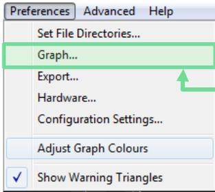
Navigate to the *Preferences* → *Graph Settings* option to adjust the current graph settings. Bin widths can be chosen separately for size, diffusion and zeta graphs, and depending on whether raw or FTLA data is used. These settings can be defined on a per Windows User Account basis.
