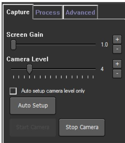
Click the *Auto Setup* button in the *Capture* tab to focus the image and set an optimal camera level for measurement
