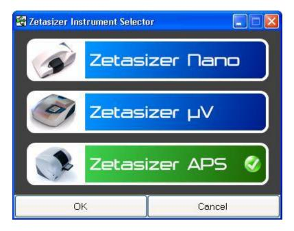
The instrument type can be changed at any point by selecting the menu item; 'Tools', 'Options', 'Instrument type'. Once the instrument type has been changed the software must be restarted for the change to take effect.
