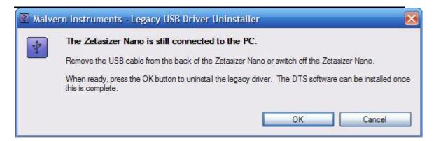
You must either switch-off the Zetasizer Nano or unplug the USB cable from the PC or Zetasizer Nano and then press OK. If you press the Cancel button the installation will continue but the legacy USB driver will not be uninstalled.
