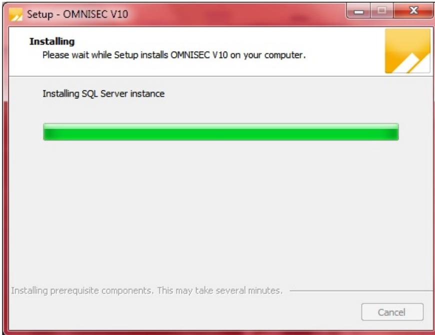
If this is the first time OMNISEC v10 is being installed, it will install a 2014 SQL Server instance. This process may take 10 to 20 minutes to complete.
