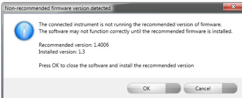
Updating the firmware improves system reliability and compatibility with the version of OMNISEC V10 you have installed on your computer. The update process takes up to 10 minutes and the instrument will need to be power cycled after the update is complete.
