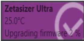
*Figure 4 instrument firmware updating status icon*
