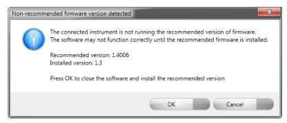
Updating the firmware improves system reliability and compatibility with the version of OMNISEC V11 you have installed on your computer. The update process takes up to 10 minutes and the instrument will need to be power cycled after the update is complete.
