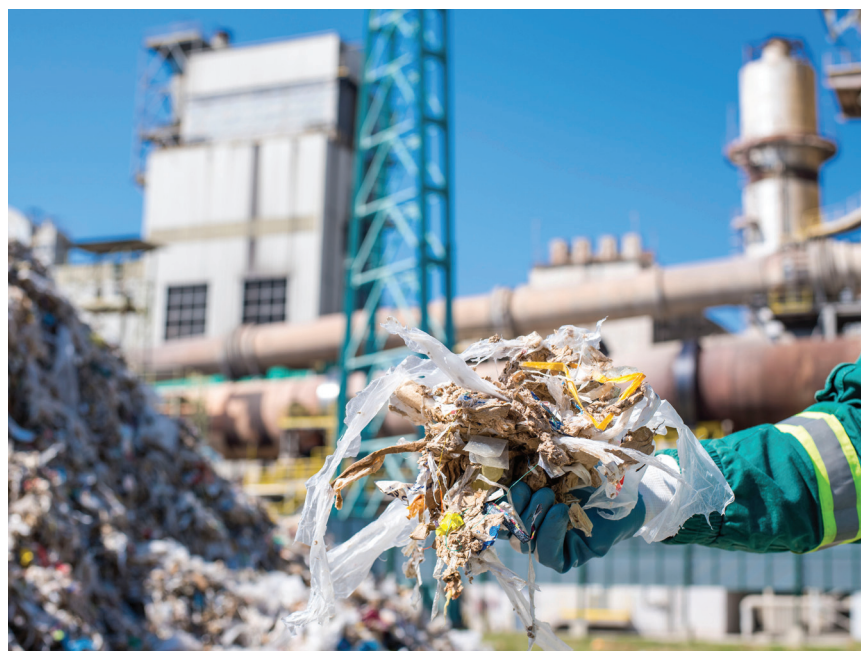
Image 2: Shredded municipal waste in front of rotary cement kiln used as alternative fuel
